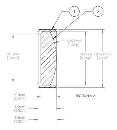
NOTES/SPECIFICATIONS: FOCAL LENGTH: 50.0mm ±1% WORKING DISTANCE: 44.2MM WAVELENGTH RANGE: 350nm-2.0µm
