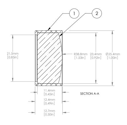
NOTES/SPECIFICATIONS: FOCAL LENGTH: 75.0mm ±1% WORKING DISTANCE: 66.4mm WAVELENGTH RANGE: 350nm-2.0µm DESIGN WAVELENGTH: 587.6nm CLEAR APERTURE: >21.0mm
